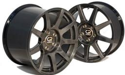
Our main presentation will be from Jake Dingle of Carbon Revolution, being the first company in the world to commercialise a one-piece carbon fibre composite wheel for the automotive industry. The first commercial production line will be commissioned in 2012.
